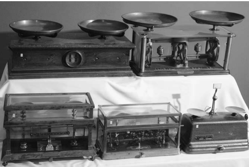
Marble top wood Troemner, all-glass torsion, all-metal torsion, steel-framed torsion, and Elmer Grimm Sr.'s wood-framed torsion
