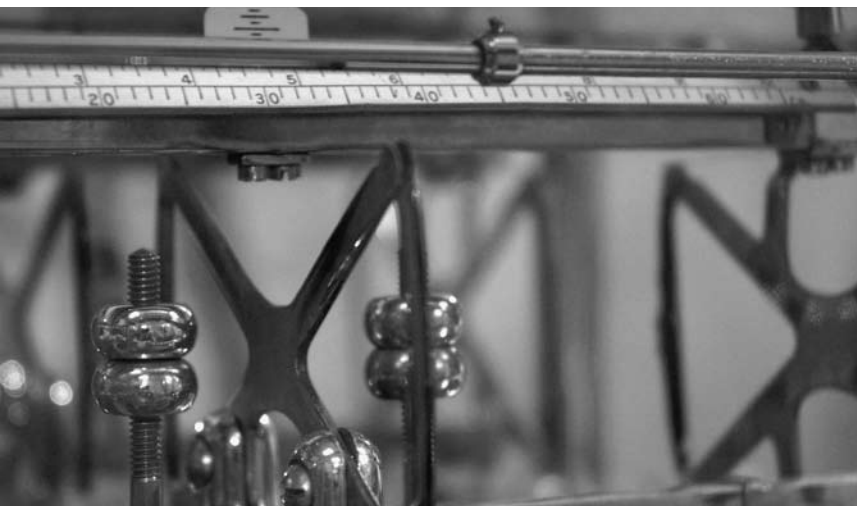
Torsion balance's factory adjustment screws and grains/milligrams weight slide gauge
